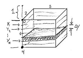
Then layer # k must be pumped a distance of approx. 1+yk meters.
