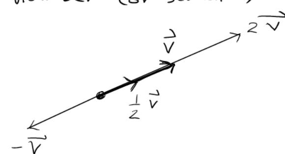
Thus  $k\vec{v}$  is just  $\vec{v}$  scaled by a factor of  $k$ . Vector  $k\vec{v}$  is called a "scalar multiple" of  $\vec{v}$ .
