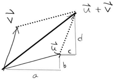
Geometrically,  $\vec{u} + \vec{v}$  is the diagonal of the parallelogram formed by  $\vec{u}$  and  $\vec{v}$ . This is true for vectors in 2-D as well as in 3-D.
