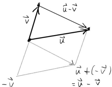
Geometrically,  $\vec{u} - \vec{v}$  is the vector directed from the tip of  $\vec{v}$  to the tip of  $\vec{u}$ , as illustrated.
